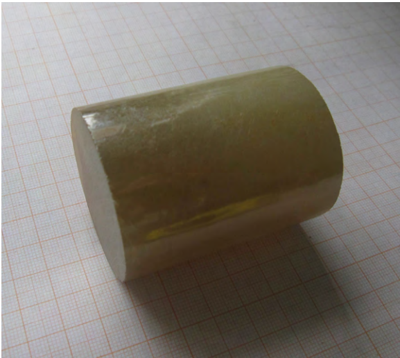
Fig. 1. A photo of 0.23PIN–0.45PMN–0.32PT single crystal with 50 mm diameter.
